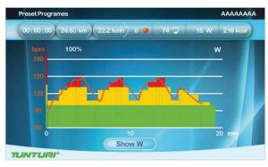
The X-axis unit is shown according to the selection of Time/Distance in Set screen:
