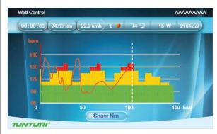
The X-axis unit is shown according to the selection of Energy/Time/Distance in Set screen.
