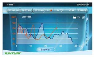
The X-axis is shown as distance unit, km in metric and mile in Imperial
