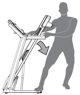
9. Grasping the Side Handrail and the front of the Upright, safely roll the treadmill to the desired location.
