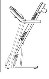
7. Make sure that the locking mechanism is engaged. Carefully pull back on the Walking Deck and make sure that it does not move. When you do this, keep clear of movement path in case the treadmill lock is not engaged.
