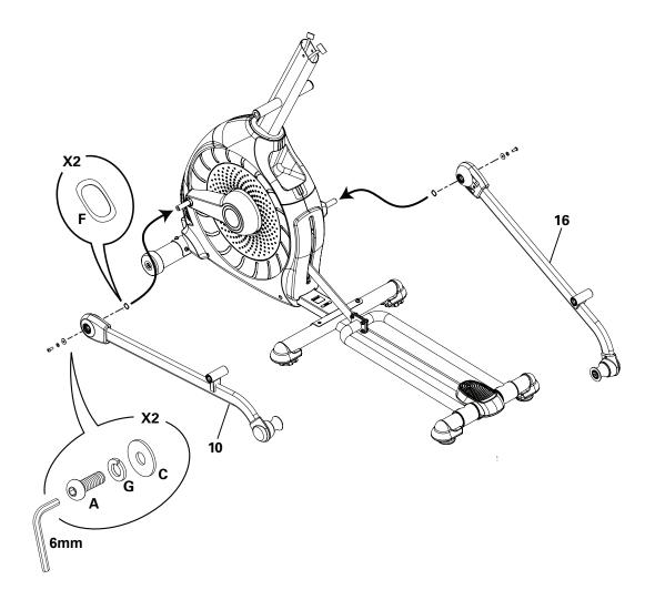
5. Attach Arm Pivot Rod and Lower Handlebar Arms to Frame Assembly
