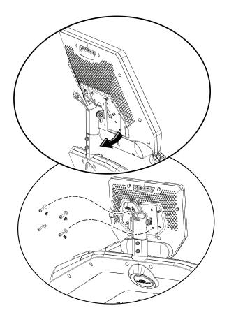
a. Place the Console onto the Console Mast and route the Cables through and out of the Console Mast
