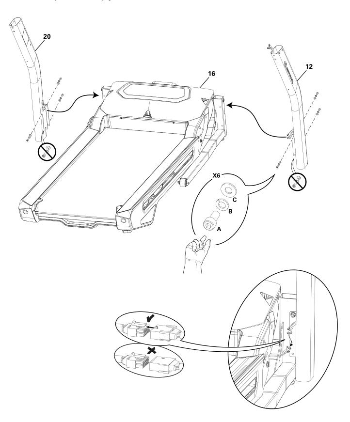
2. Attach the Crossbar and Pivot Shrouds to the Frame Assembly
